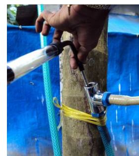
Figure 18: “Three ways installed to carry out the \text{CO}_2 measurements.
