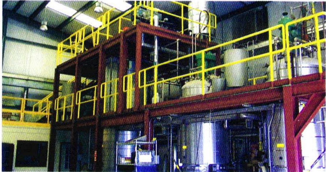
Large-scale TVA facility in Muscle Shoals, Alabama processes biomass feedstocks such as sorted municipal solid waste and agricultural residues into fermentable sugars, which are converted into ethanol.
