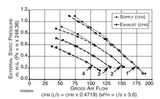
SPEED RANGE\* 1: 80 TO 157 CFM SPEED RANGE\* 2: 66 TO 132 CFM SPEED RANGE\* **3**: 53 TO **106** CFM SPEED RANGE\* 4: 40 TO 80 CFM \* AT 0.4 IN. W.G.
