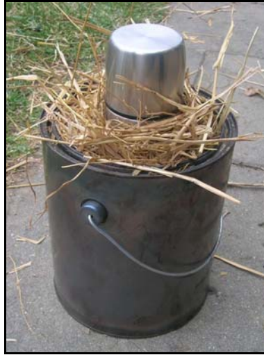
Figure 2. Packing wheat straw around a central cylinder.
