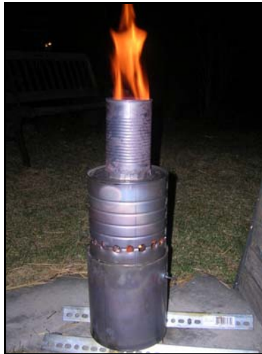
Figure 5. Bottom-lit, hollow-core straw just after ignition. The gas fire died down and burned to completion after 10-13 minutes.
