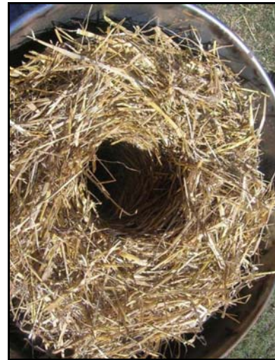
Figure 9. Hollow-core bed of compressed wheat straw in the drum gasifier.
