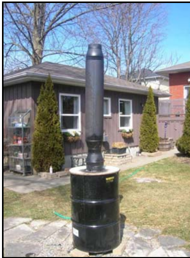
Figure 8. Nested drum gasifier with a venturi afterburner.
