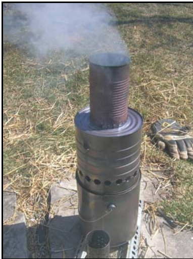
Figure 4. Top-lit, hollow-core straw – the gas fire went out before all straw volatiles had gasified.
