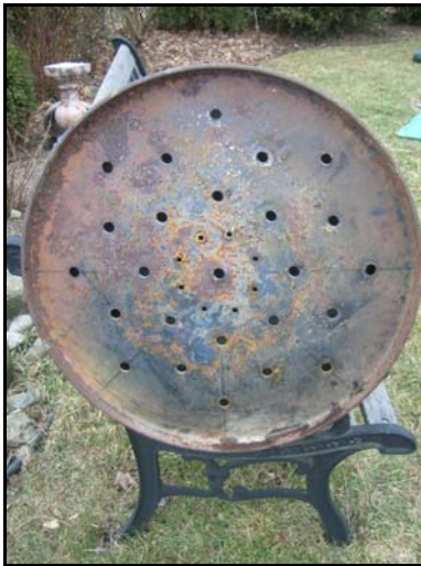
Figure 7. Primary air holes in the bottom of the 118-L drum.
