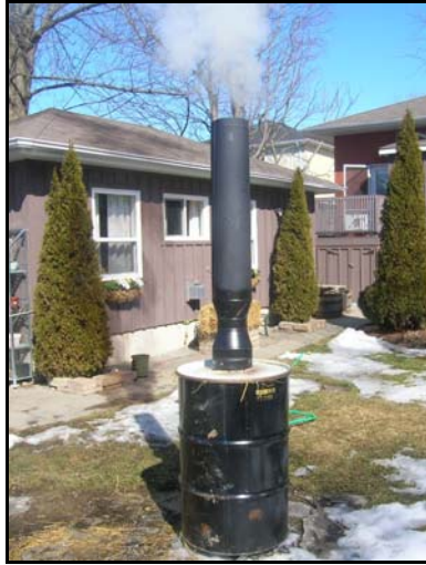
Figure 10. The gas fire above top-lit, loosely packed, solid bed of straw went out two minutes after ignition, and smoked for three hours.
