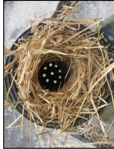
Figure 3: Hollow-core packed straw with primary air holes visible at the bottom.
