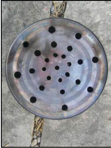
Figure 1. Primary air holes in the bottom of the paint-can gasifier.
