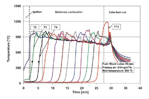
The temperature of the fuel bed rose from room temperature to about 800-900 °C as the ignition front moved downwards. The charcoal above the ignition front remained at about that temperature. After about 28 minutes, the ignition fire had reached the bottom of the reactor and a charcoal fire remained (as shown by a sharp rise in the temperature of bottom thermocouple, T13).
