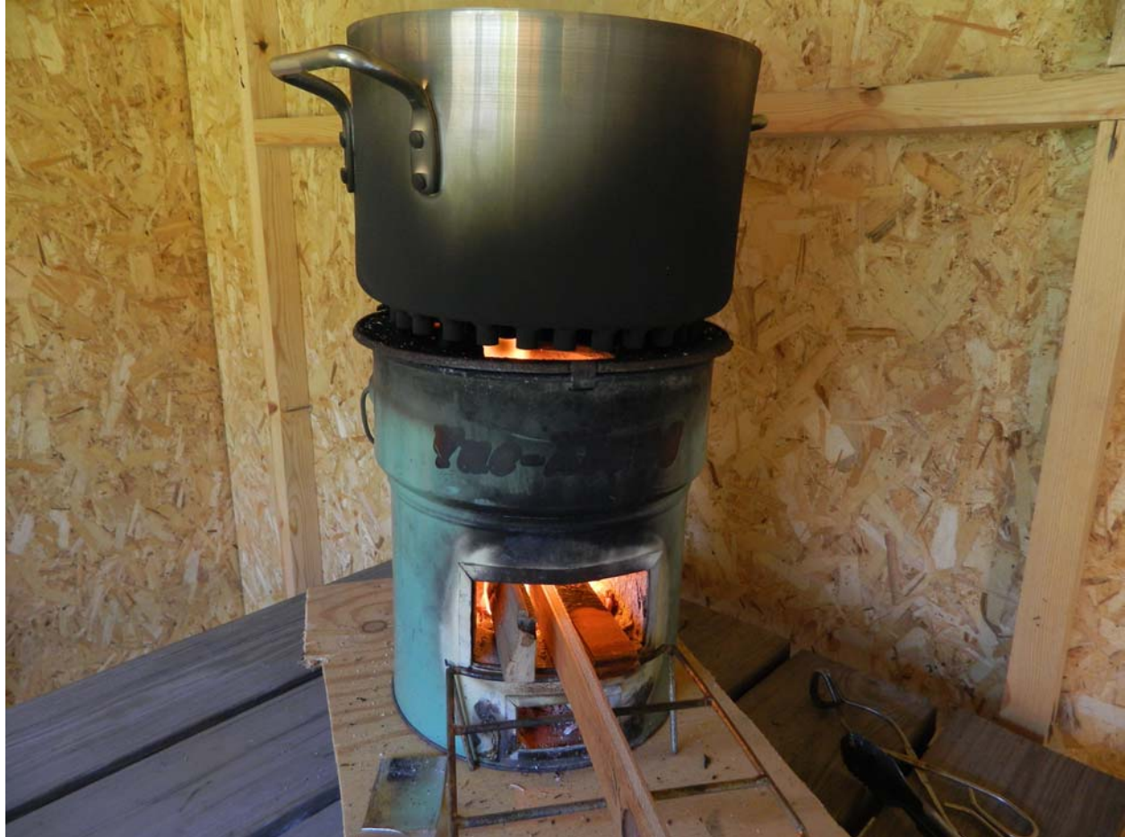
Figure 4: The ceramic rocket stove with the finned pot, using wood as the fuel.
