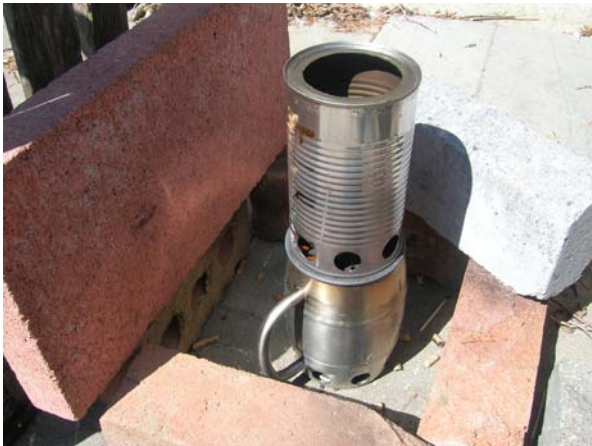
Fig. 1: A chimney over the cap with holes for secondary air improves combustion if the gas fire penetrates the holes in the cap.
