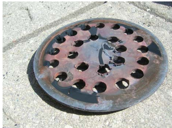
Fig. 4: Underside of cap after the burn in Fig. 3. Soot deposits are black patches, especially at the top-left.
