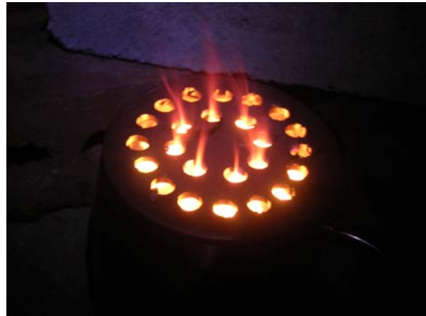
Fig. 2: With maximum primary air, the gas fire penetrates the cap, with incomplete combustion producing a small amount of smoke
