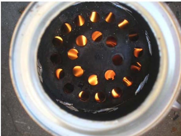
Fig. 3: Gas fire confined and swirling under the cap, by cutting back on primary air. No visible smoke.
