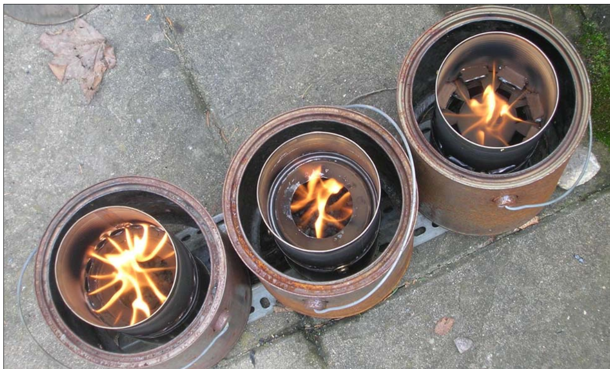
Figure 3. Flame structure for ConcBelow, ConcAbove, and Rectangular syngas burners.
