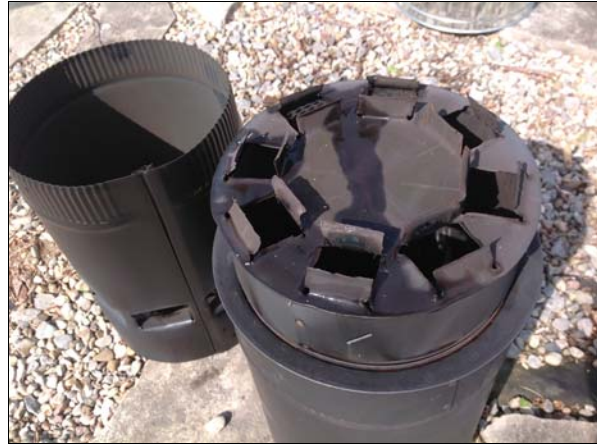
Figure 2. Discontinuous annular burner on top.
