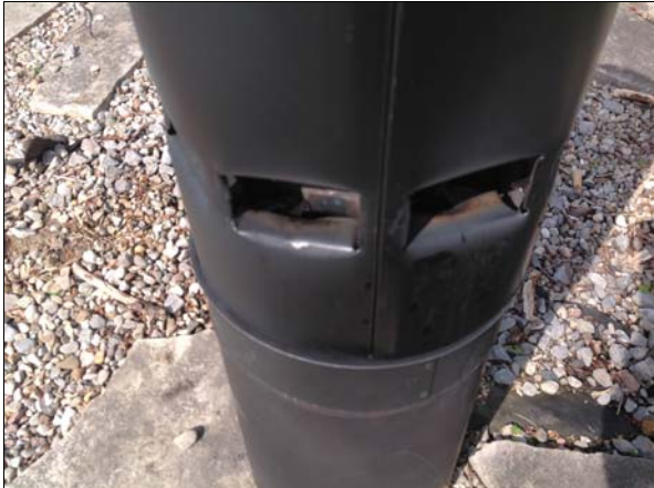
Figure 3. Chimney with secondary air holes.
