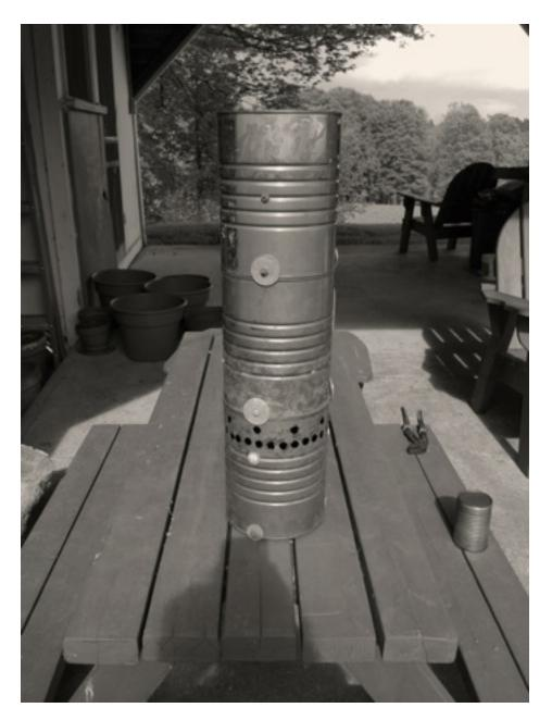
The final draft enhancing can has been added to complete the system. You can see the use of three small washers to create the air gap for the secondary air. Three larger washers at the base of the other cans helps to lock them into position and to prevent them from falling off the stack. Note also the 3/8th inch secondary air holes. The bottom rings has 29 holes and the top rings has 9. I find that multi level secondary air works better than a single layer.
