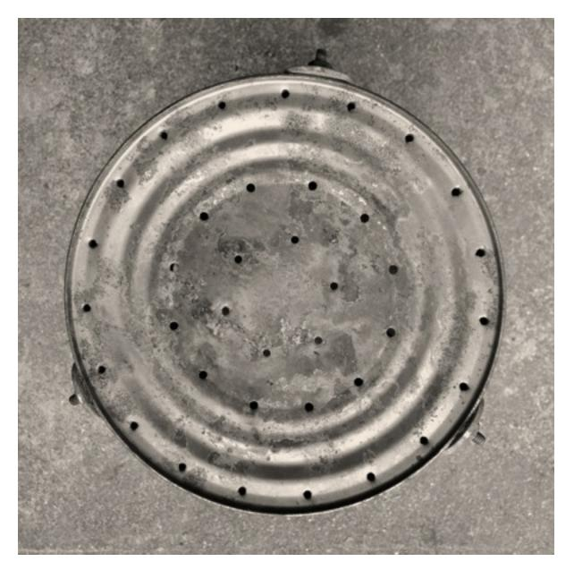
The bottom of the reactor can. The primary system is set up for dry wood pellet fuel. It can be modified to work with other fuel types. Ideally, the primary system would be on a plate that could exchanged as power levels and fuel types required. Increasing the primary air, for example, will create a hotter & faster pyrolysis if heat is the primary goal.
