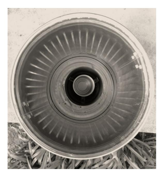
The above two photos show the natural draft iCan TLUD configured to boil water in the Swiss Volcano Stove manner: pot set into the exhaust gas stream with thermal energy applied to the sides and bottom of the water container.
