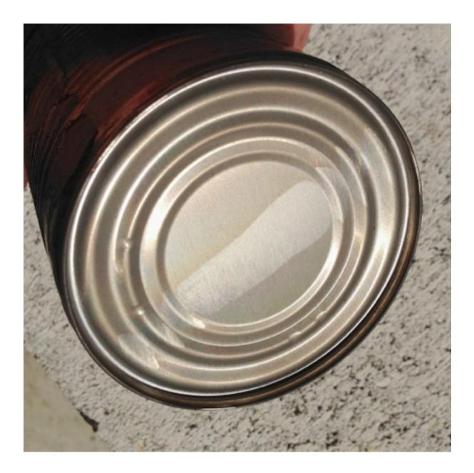
In a well tune iCan TLUD, very little soot will be deposited on a "pot" used to boil water. The "haze" on the bottom of the can above is mostly a light varnish of creosote that washes off easily. Soot on pot bottoms indicates incomplete combustion of the the carbon monoxide in the syngas. For the most efficient use of the syngas, soot should be avoided.
