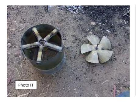
This photo shows the 5 pipe arrangement used on the stove that first passed the ISO-IWA low power tests. This arrangement is difficult to build, so it was important to find how to get the much simpler single pipe arrangement to work. The 5 pipe design uses 5/8" (2 cm) ID pipe with 3/16" (.4 cm) wide slots. The single pipe arrangement uses 7/8" (2.3 cm) ID pipe with 5/16" (.7 cm) wide slots.
