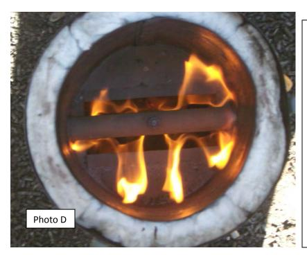
This photo shows the flame with the stationary fan removed for clarity. The flame is coming toward us, out of the picture. It emerges from below the edges of the rectangular concentrator hole and approaches the pipe as it rises. It then curves away from the pipe, blown by the air from the pipe. Looking through the wall of the combustor from the end of the pipe, the flame pathway would look like
