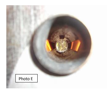
This is the view looking into the end of the pipe. Visible are the slots and the flames passing the slots. The screw in the top of the pipe holds the stator fan and the deflector. At the very center are the plants in the background, visible because we are looking through the pipe which is open at both ends.
