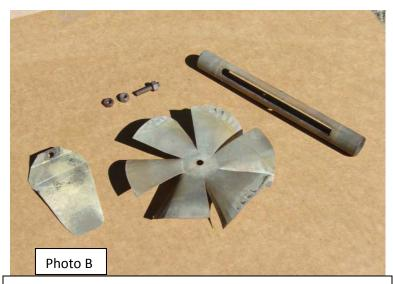
Here is the pipe with slots laid out for clarity. The fan and deflector are explained below. The parts are designed to fit into a 6'' (15 cm) diameter inside wall by 8'' (20 cm) outside wall combustor. The fan diameter is 6'' (15 cm) and the pipe is  $8 \frac{1}{2}''$  (21.5) long with two  $5 \frac{3}{4}''$  (14.5 cm) slots. The fan is 1'' (2.5 cm) above the pipe which is 1'' (2.5 cm) above the concentrator ring.
