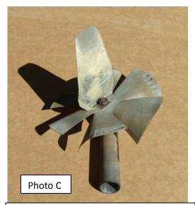
Here the pieces are assembled as they will be inside the combustor. The flame rises past the pipe, then the fan and then the deflector. Two of the stationary fan blades are located directly over the pipe to give the best results.
