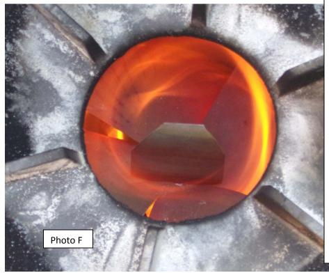
This photo shows a flame of about 5 kw contained in a 7" (18 cm) tall by 6" (15 cm) inside diameter combustor. It is traveling about ¾ of a revolution around the combustor. Note the metal inside the combustor is red hot from the concentrated flame. The deflector, which keeps the flame out of the center, is foreshortened in this view. The white on the pot holder is the ash from burned paint. This was a test of a four bladed fan, but I have found that 6 blades seem to work better.
