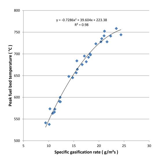
The quadratic regression ( $R^2 = 0.98$ , AIC = 212) was a significant improvement (p < 0.001) over a linear regression ( $R^2 = 0.95$ , AIC = 240). Gaps in the distribution of points result from the choice of grate apertures.
