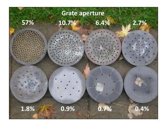
(NOTE: The arrangement and diameter (4.76 mm) of holes affects air flow and may yield slightly different power curves than other methods for air control. The "57%" was a wire mesh. This method has helped to reduce channelling of the pyrolytic front in wood chips, and was repeatable.)
