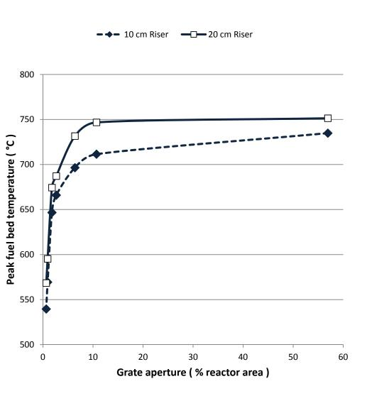
Increasing riser height significantly ( p < 0.001 ) increased temperature.
