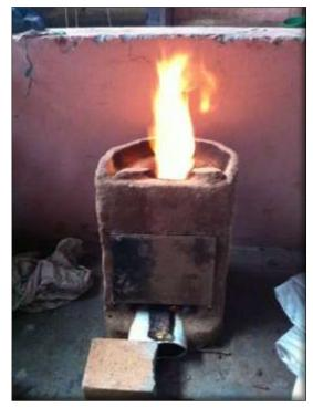
The primary air enters through 25 holes about 0.6 cm in diameter, evenly spaced across the bottom of the fuel canister. Secondary air enters near the bottom of the fuel canister under the door (area is about 50 cm<sup>2</sup>) and
