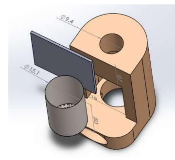
through a hole in the back (about 30 cm<sup>2</sup>). This air rises through a 1 - 2 cm wide space between the can and the stove body and then is forced through a 1 cm wide gap at the top of the canister where it mixes with the wood gases. The ratio of primary to secondary air supply is approximately 1 to 6 by surface area.
