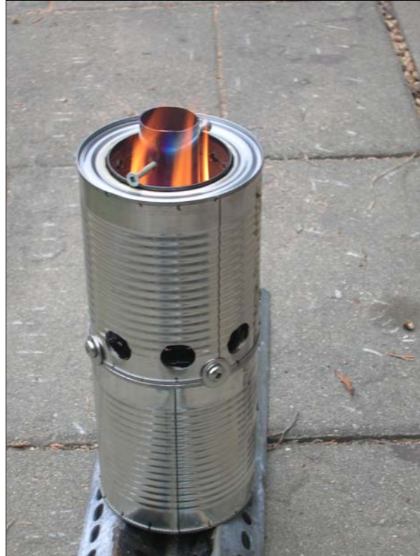
Figure 6. At a high gasification rate, the flame exited the burner. The cooling flame above the burner emitted soot coming from the flame tips. Gas combustion may be complete if the burner was taller.
