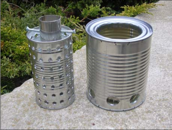
Figure 5. Perforated cylinder (open top and bottom) containing a gas wick to position the flame close to the cylinder side walls.
