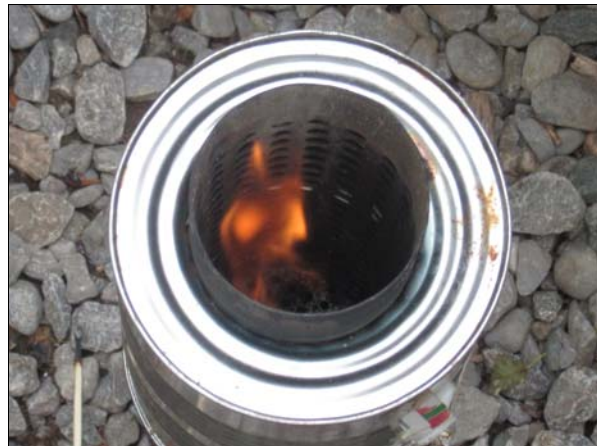
Figure 4. High gasification rate: A tall yellow gas flame forms up the central axis of the burner, and extended 0-10 cm above the top of the burner. Some soot was observed at the top of the flame, even if the flame was within the burner. The gas flame was forced away from the edges of the cylinder by entering secondary air. Entrainment of secondary air into the flame is imperfect, and it is likely that a substantive quantity of the air exits the burner unreacted.
