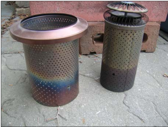
Figure 7. Outer (hollow) (99 mm diameter) and inner cylinders (76 mm diameter, enclosed top and bottom)
