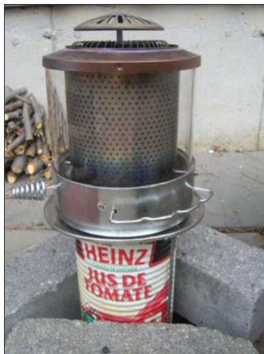
Figure 7. Outer (hollow) (99 mm diameter) and inner cylinders (76 mm diameter, enclosed top and bottom)
