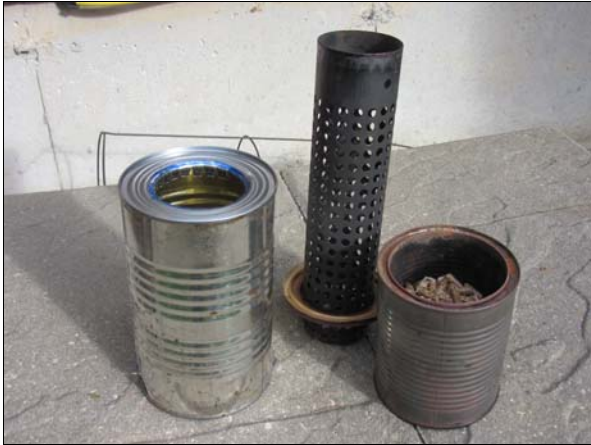
Figure 1. From left to right: (a) burner shroud for pre-heating secondary air, (b) perforated cylinder with open top and perforated bottom, and (c) ND-TLUD reactor.
