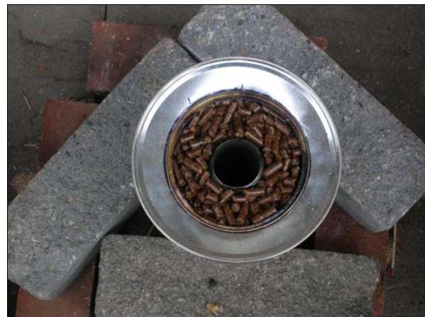
Figure 8. Inner cylinder nested inside the outer cylinder, forming an annular combustion space for produced gas.
