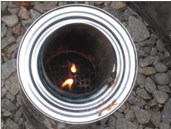
Figure 3. Low gasification rate: Small, stable flamelets formed at the bottom of the cylinder. This burner was able to support low turn-down of the gasification rate. It is possible that a substantive amount of unreacted air entered through the holes above the flame.
