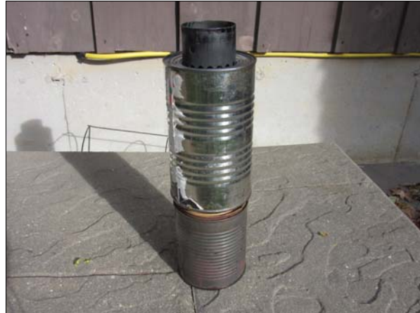
Figure 2. The assembled ND-TLUD ready for lighting. Secondary air enters through a gap between the top of the reactor, and the bottom of the burner shroud.
