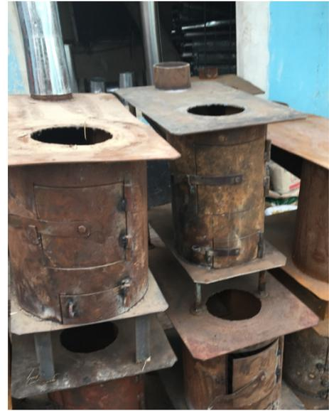
Figure 1: The locally made stove with the long horizontal chimney tested with wood and then coal.
