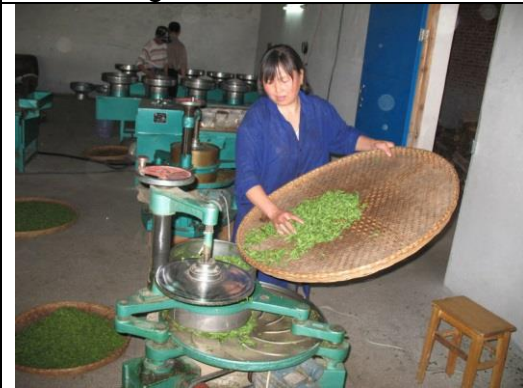
Tea roaster on the back (feedstock adding place) and front (roasting turning drum)
