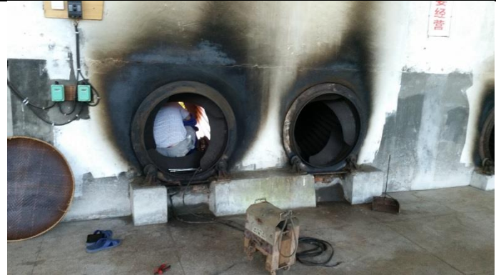
Tea roaster on the back (feedstock adding place) and front (roasting turning drum)
