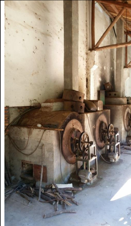
Tea roaster on the back (feedstock adding place) and front (roasting turning drum)
