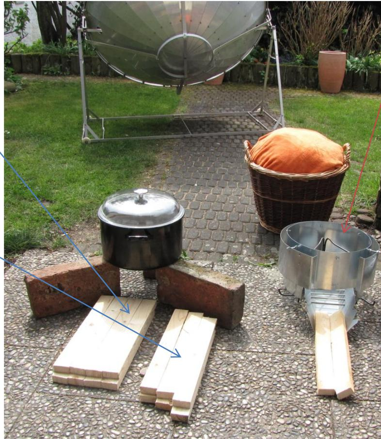
Ben-Stove needs approx. 400 g wood (small sticks) for boiling 6 liters of water (efficiency 40%). Cooking with retained heat (e.g. cooking dry beans in Thermo-Basket) is done without fuel consumption.
