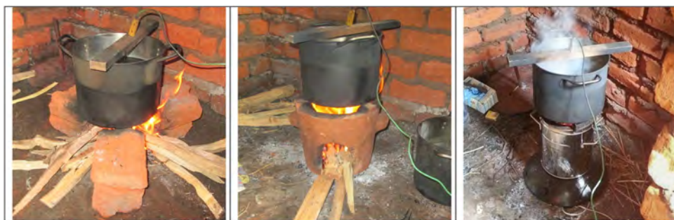
Fig. 1. Biomass burning stoves included in this study. From left to right: three-stone fire, Chitetezo Mbaula, and Philips HD4012 fan stove.
