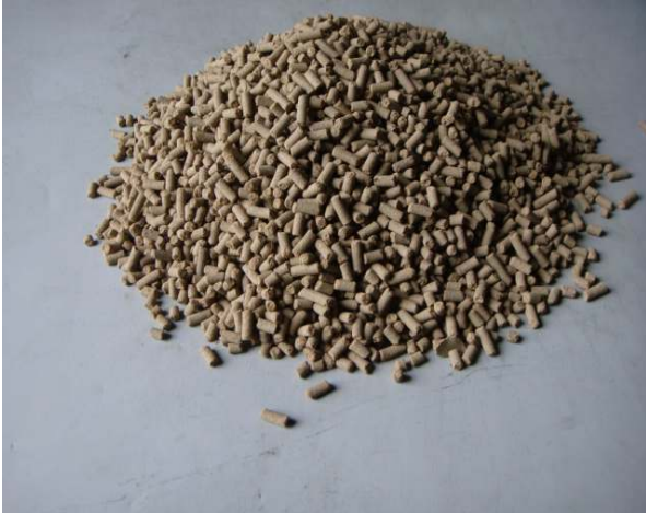
. Figure 4. Pellet produced from sawdust does not mix other types of coal burned into blue gas
