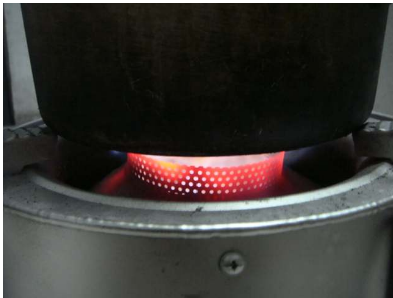
Figure 31. On the stove can create a high-temperature gas (800-900 degrees Celsius) It's as easy as the LARGE and MEDIUM!
