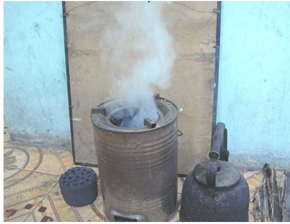
Figure 3. A modern honeycomb coal stove but still emits a lot of smoke and toxic gases
