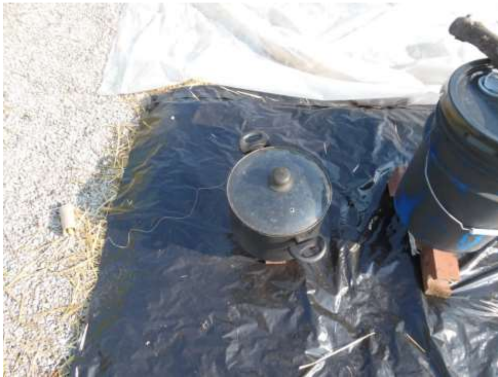
Figure 6: A cooking pot with 5 liters of water. The clear top gives the best performance, but an opaque top works almost as well.
