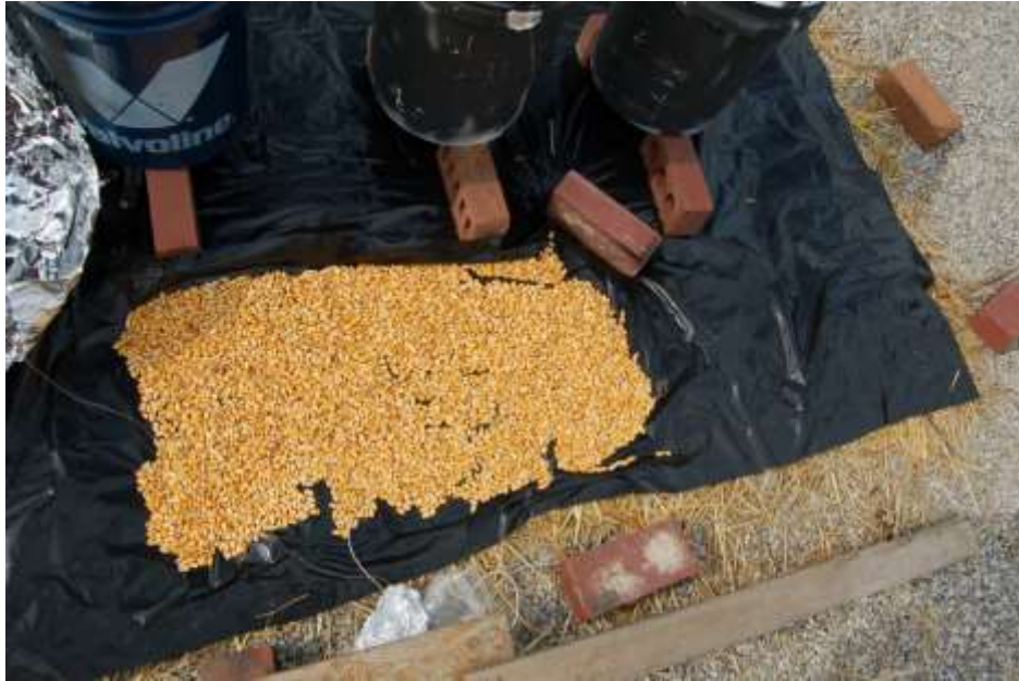
Figure 5: An arrangement showing three buckets and about 3.3 kg of corn to be dried. The layer of corn is just under 1 cm thick.
