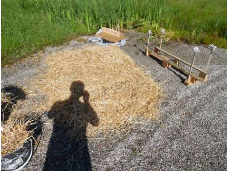
Figure 1: The straw used as the bottom insulation. It is about 5 cm thick.
