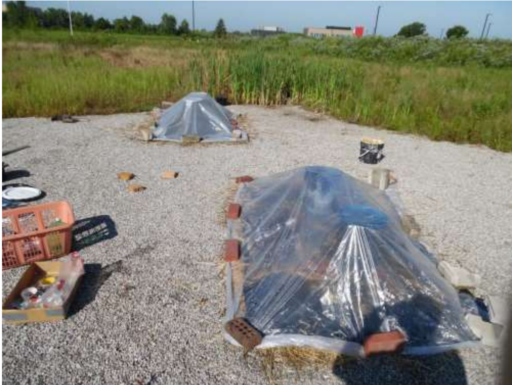
Figure 7: The test units fully set up. The near unit with the water bottles has a clear cover and the far unit with the wood to be dried has a translucent cover. Both seem to perform about equally well. The clear plastic is draped over the open tops of the buckets to allow sunlight to hit the inside of the bucket. There are no lids on the buckets.
