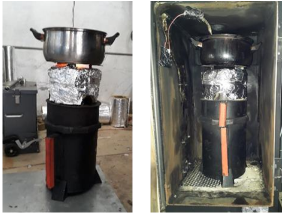
Figure 3: Picture of the setup for the water boiling test (left) and measurement of CO emissions (right) with modified Awamu cook stove and 5 litre pot (Note: the boiler door is closed during the CO emissions test).
