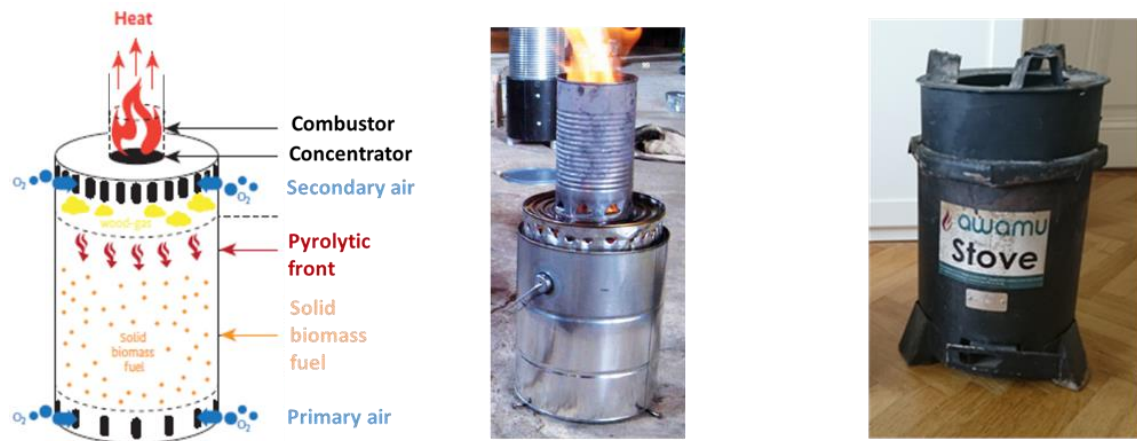
Figure 1: TLUD cook stove concept (left) and in operation (middle) [5]. Employed original Awamu cook stove in this work, based on the TLUD concept (right).
