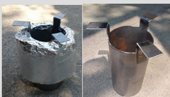
Novel combustor with and without insulation
