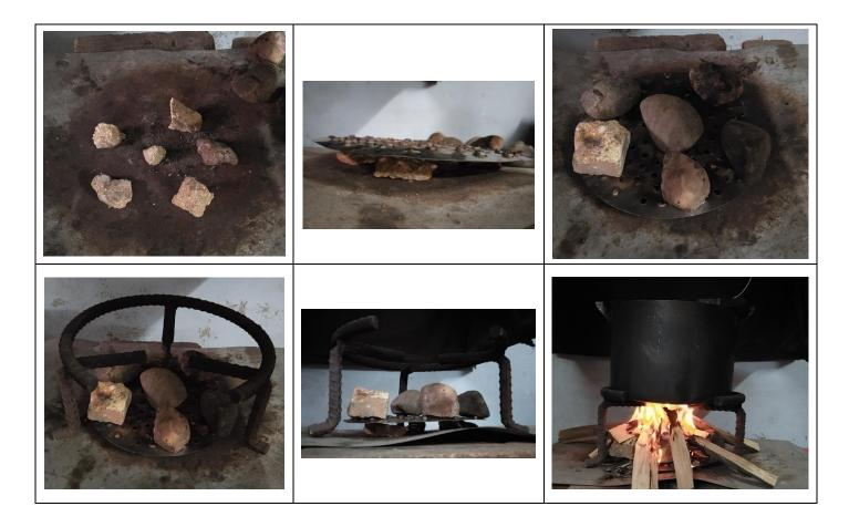
Arrangement for rocks bed IB + conical pot skirt:
